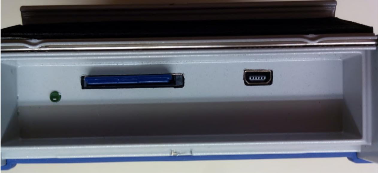
Figure shows open flap on top of the device with SD - card and USB - connection. The USB interface is necessary for update the firmware to be made. This requires a connection to a USB cable to a PC. The following figure shows the necessary cable.
